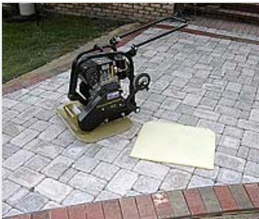
Since this project involved clay pavers, a rubber mat was attached to the bottom of the plate compactor to minimize chipping and cracking. A rubber mat is also a good tool when running the compactor on top of textured surface concrete pavers. There are also roller attachments available for this same purpose.
